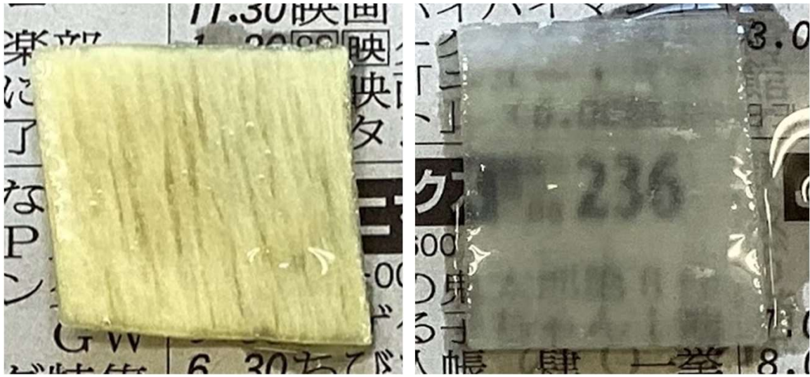
Left: Balsa 1mm processed by 0% \text{H}_2\text{O}_2\text{aq}
