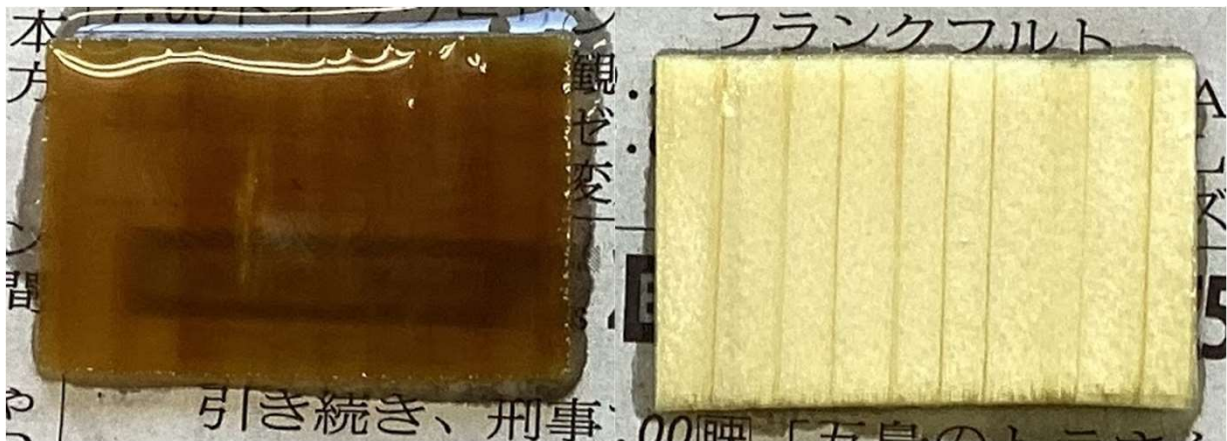
Left: cypress 1mm processed by 0% \text{H}_2\text{O}_2\text{aq}
